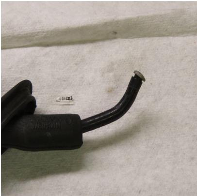
5. After a good dousing with alcohol, flatten the boot as shown in #1, and while flat...twist and push the old wire through as shown. Keep working it, it will come through. Note the tip is soldered in. I used a vise to hold the wire & heated the solder with a gun. Under that solder is nothing more than a small washer...remove it and use it on the new wire. Now pull the old wire back through the boot...may need more alcohol
