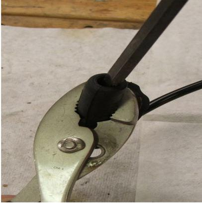
3. Unscrew the top piece (slotted for a screwdriver) by holding the internal plastic case firmly while still in the boot, but don't squeeze hard. It will come loose, but if you crack it do as I did with one...used some good plastic glue and let set overnight. It works fine. After removing the top screw-out piece, the resistor will drop out. Remember, the plastic case doesn't have to be removed.
