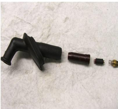
2. This shows the “innards” of the boot. The internal plastic case doesn't have to be removed, the rubber sleeved item in the center is the resistor, the item on the right with the spring is the part that screws out of the plastic case (careful to not lose the spring).
