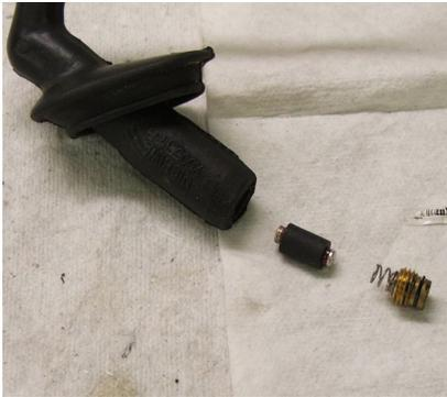
4. This is all that needs to be removed. After this, you will be able to push the old wire through from the "coil" side of the boot
