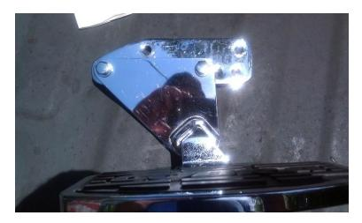
The Rattlebars shifter is curved at the rear to clear the Valk's exhaust system but the Wing shifter is flat at the rear. I used 1/4 inch spacers between the peg mounts and the Peg Relocation Plates.
