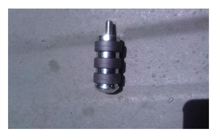
First I cut off the shock shift peg, then drilled two holes in the shift arm and tapped them. I drilled the first hole in the stock location and the second hole halfway down the shift arm. I did this so I wouldn't have to disassemble everything if I didn't like where the shift peg was at then drill/tap another hole.
