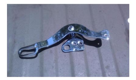
First, I removed the pivot bolt as it is also the bolt that mounts the shifter to the mounting plate.
