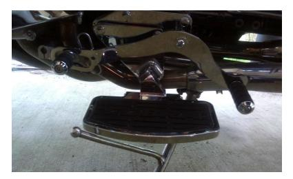
After a few teething problems getting it adjusted, it has been problem free on my Interstate since June, 2012. I discovered using the forward mounting hole for the front shift peg allowed me to have a more natural foot position. Using the rear mounting hole required me to angle my foot about 45\*.
