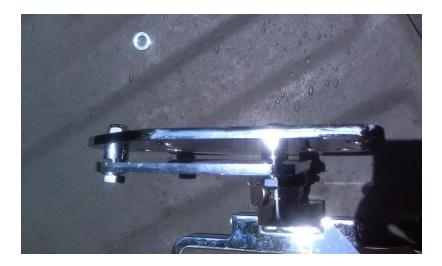
I discovered the mounting/pivot bolt wasn't long enough to go through the Peg Relocation Plate, so I replaced it with a polished stainless steel button head bolt, washer and nylok nut I bought at Ace Hardware. The shifter has a washer between it and the mounting plate. It acts as a spacer for the shifter's bushing so I installed it between the shifter and the Peg Relocation Plate then bolted the shifter to the rear bottom hole in the Relocation Plate.
