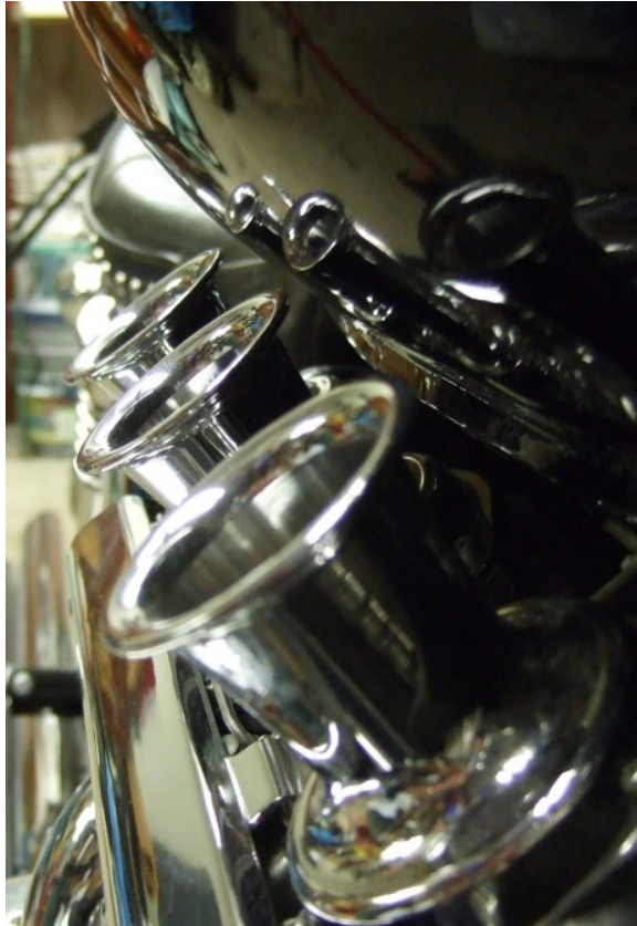
Picture shows the minimal clearance with a ½ inch spacer installed.
