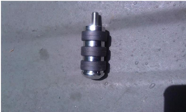
First I cut off the shock shift peg, then drilled two holes in the shift arm and tapped them. I drilled the first hole in the stock location and the second hole halfway down the shift arm. I did this so I wouldn't have to disassemble everything if I didn't like where the shift peg was at then drill/tap another hole.
