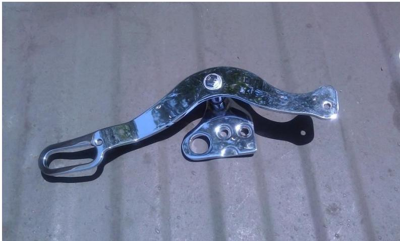
First, I removed the pivot bolt as it is also the bolt that mounts the shifter to the mounting plate.
