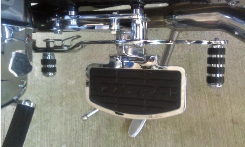
As you can see the heel/toe shifter and stock shift arm rubbed so I replaced the spacers between the frame and plate with 1/2 inch spacers. I installed a Kury Longhorn ISO Shift Peg at the heel position then used a washer and nylok nut to secure it. I also added a washer and nylok nut to the front Kury peg to make sure it stayed on.
