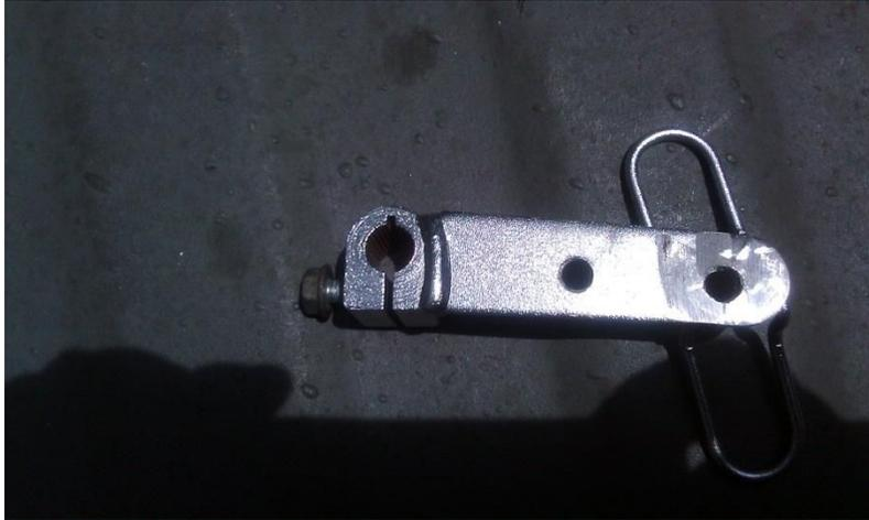
I attempted to insert the Kury peg through the slot in the shifter but the peg was too big. I removed the inner post and sanded the inner end with a Dremel tool until it fit.
