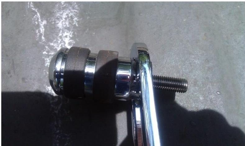
I installed the modified shift arm then the peg assembly with the heel/toe shifter and bolted the Kury peg to the forward hole in the shift arm. I used 1/4 inch spacers between the frame
